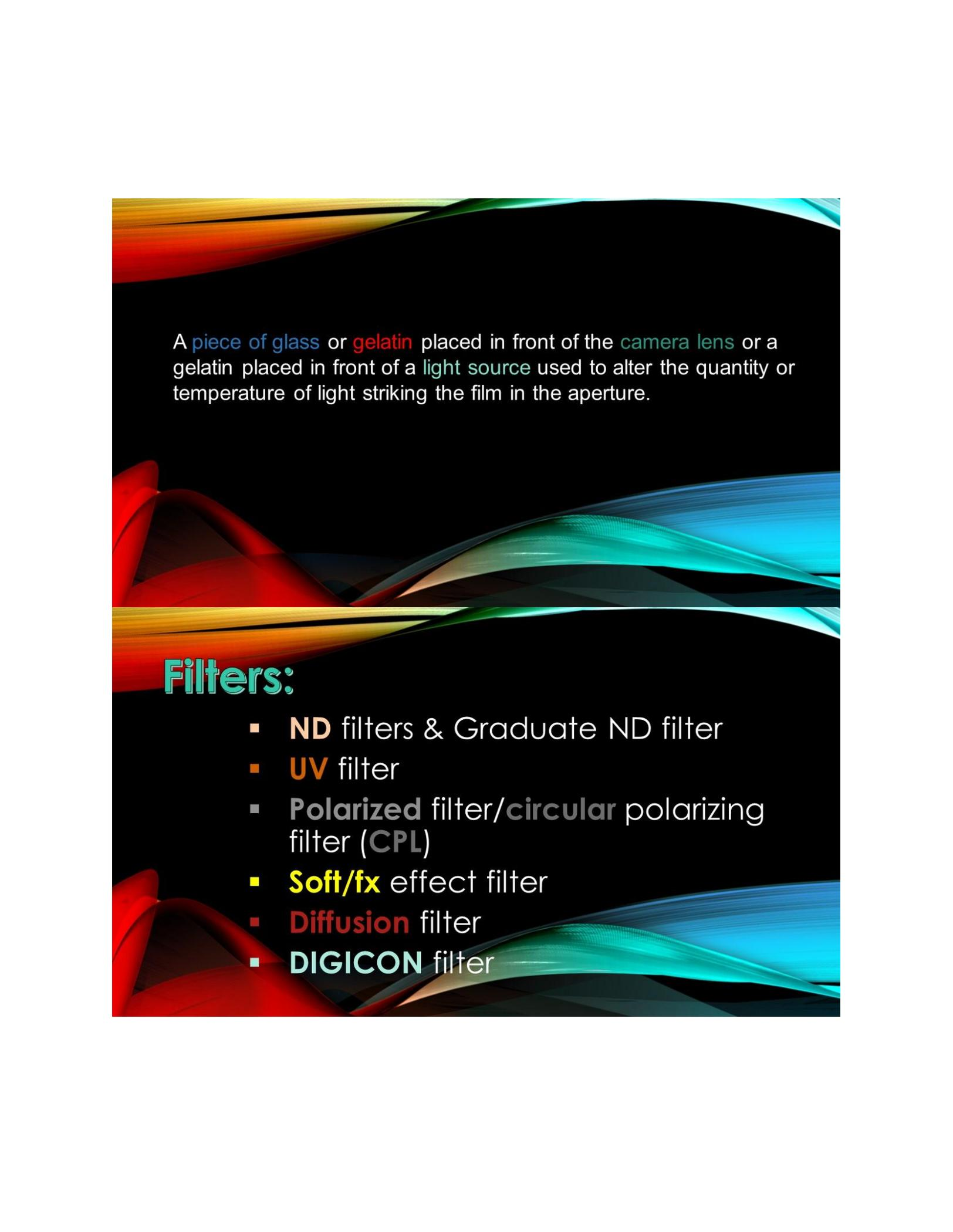
A piece of glass or gelatin placed in front of the camera lens or a gelatin placed in front of a light source used to alter the quantity or temperature of light striking the film in the aperture.
